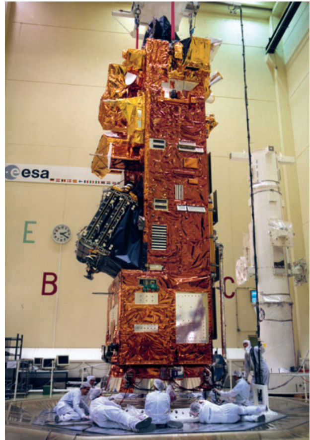
Fig.3-14: ENVISAT integration on the ESTEC Hydra vibration test facility. The instruments are covered with MLI. SCIAMACHY is the only instrument located on the front panel (top right corner). (photo: ESA)
