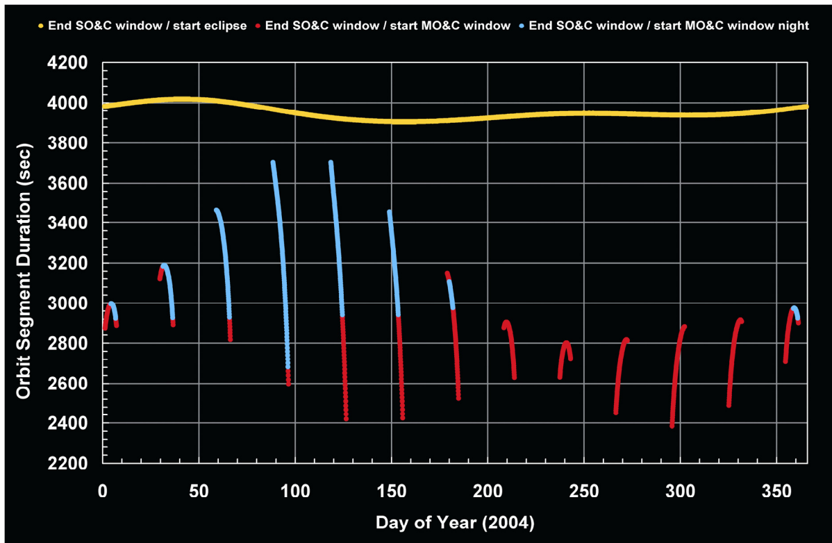
Fig. 4-11: Example of the seasonal temporal variability of orbital segments for the year 2004. The time interval between end of SO&C window and start of eclipse varies only slightly over a year (yellow). In the monthly lunar visibility periods, the time between end of MO&C window and start of eclipse shows a much higher variation (red curves). The blue segments indicate lunar visibility phases where moonrise occurs on the nightside, i.e. those which can be used for occultations. (Courtesy: DLR-IMF)
