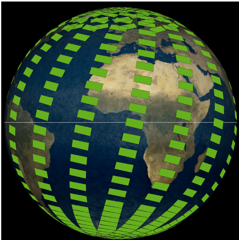
Fig. 4-7: SCIAMACHY reference orbit with Sun/Moon fixed events along the orbit. The events define orbital segments which are filled with timelines. State duration is not to scale. (Courtesy: DLR-IMF)
