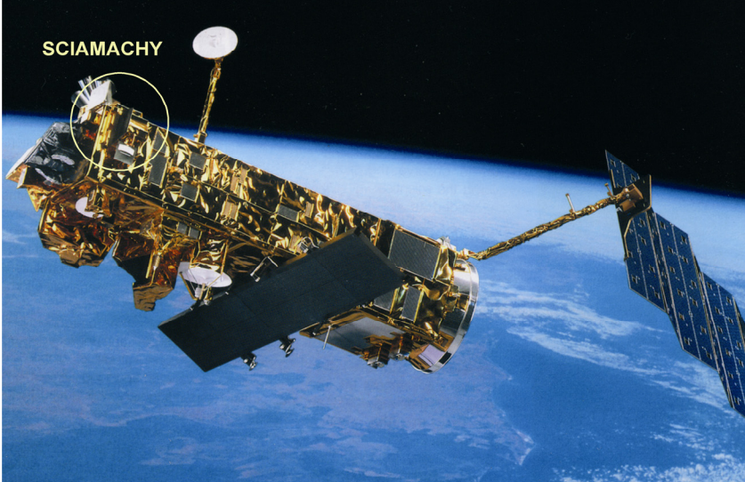
Fig. 2-1: Artist's impression of ENVISAT in orbit. SCIAMACHY is located at the upper right corner of the payload front panel. (Photo: ESA)
