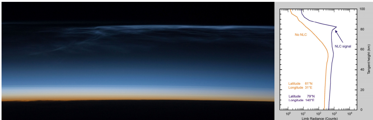
Fig. 10-30: NLC as seen from the International Space Station on 22 July 2008 (left panel), together with the NLC signature in a SCIAMACHY UV limb radiance profile from 3 July 2002 (right panel). The scattering by ice particles in the NLC leads to a significant increase of the observed limb radiance profile peaking at the characteristic NLC altitude of about 83-85 km (blue line). For comparison, a limb radiance measurement in the absence of NLC is shown in red. (Courtesy: C. von Savigny, IUP-IFE, University of Bremen; ISS photo: NASA)
