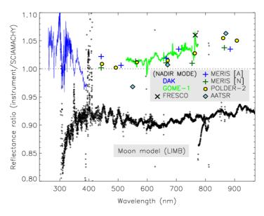
The lunar calibration results were essential in providing direction for further investigations into calibration key data improvement. The figure below shows preliminary results for the new radiometric calibration, where the ratio with a scaled lunar spectrum is shown for the old (blue) and the new (black) key data. The reduction in spectral features is obvious, and is visible due to the fact that the spectral features of the Moon are smooth, typically several hundreds of nm wide.
