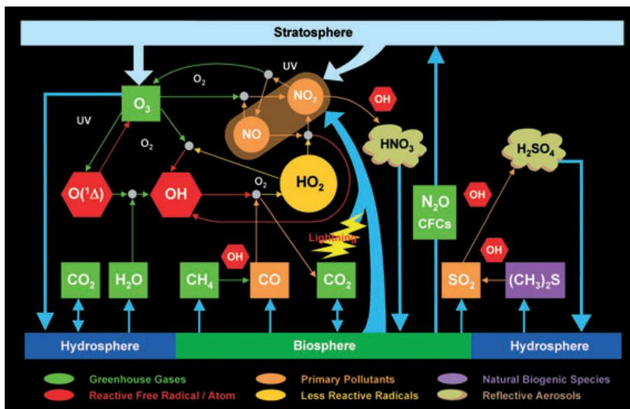
Fig. 1-4: The dominant physical and chemical processes determining the composition of the troposphere. (graphics: WMO-IGACO 2004)
